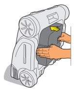
1.4.3 - Reposition the filter canister by pressing simultaneously both tabs while pushing the canister inside in the robotic cleaner until the stop, and then release the tabs to lock it in place.
