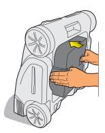
4.8.3 - Reposition the filter canister by pressing simultaneously both tabs while pushing the canister inside in the robotic cleaner until the stop, and then release the tabs to lock it in place.
