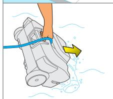
3.4 - Grab the robotic cleaner by the top handle. Put it into the pool. Release the Robotic cleaner and let it sink to the floor of the pool. Make sure that the floating cable is free of any obstructions.
