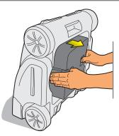
4.2 - Insert your hands in each side of the filter canister and simultaneously press both tabs to release the canister. Pull the Canister out and place it on a flat ground. Debris is stored in the canister underneath the filter.
